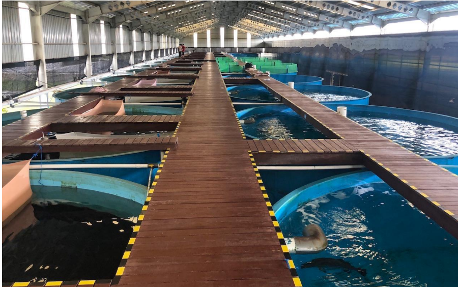
Image 2. Brood fish tanks in the Aquaculture Research Center (ARC). Each tank is 3 meters deep and 6 meters in diameter, arranged in a continuous series. These tanks are designed to produce high-quality eggs from important aquaculture species.
